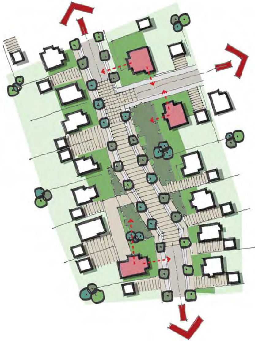
Diagram: Typical plan of a primary 'gateway' road junction
