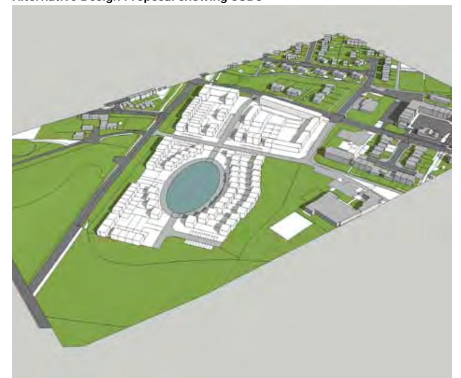
3D model of Alternative Design Proposal showing SUDS
