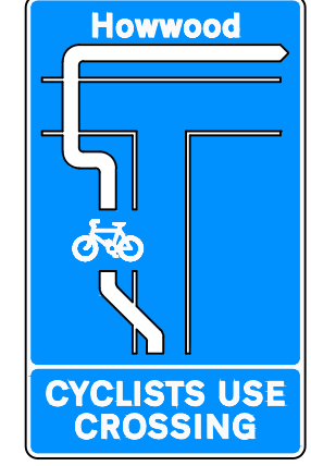
FIGURE 1: Example of map type signs to be used throughout the route at key intersections to inform cyclists of manoeuvre / transition required.
